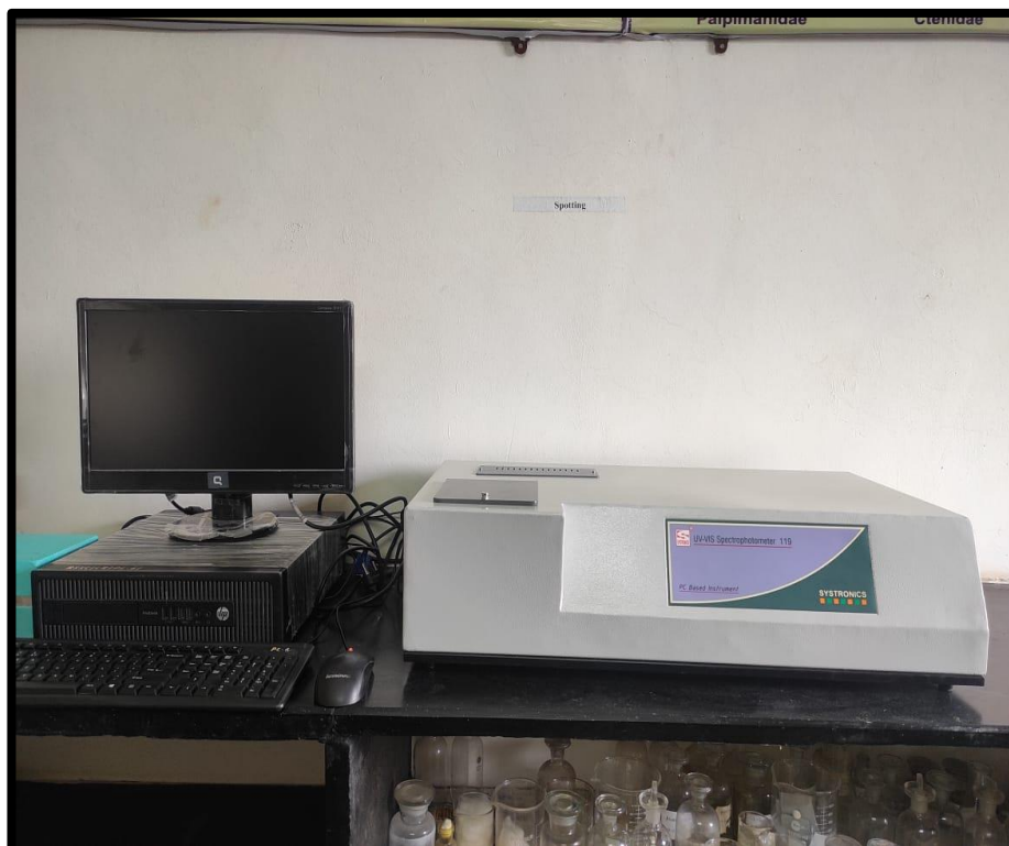
PC based visible spectrophotometer, Department of Zoology
